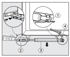
■ Using a screwdriver, carefully push tension spring ① outwards.
